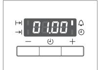
When the time has elapsed, the function indicator flashes and an audible signal sounds for 2 minutes.
